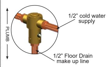
The Priming valve must have a min. elevation of 12" (305mm) above the finished floor.
